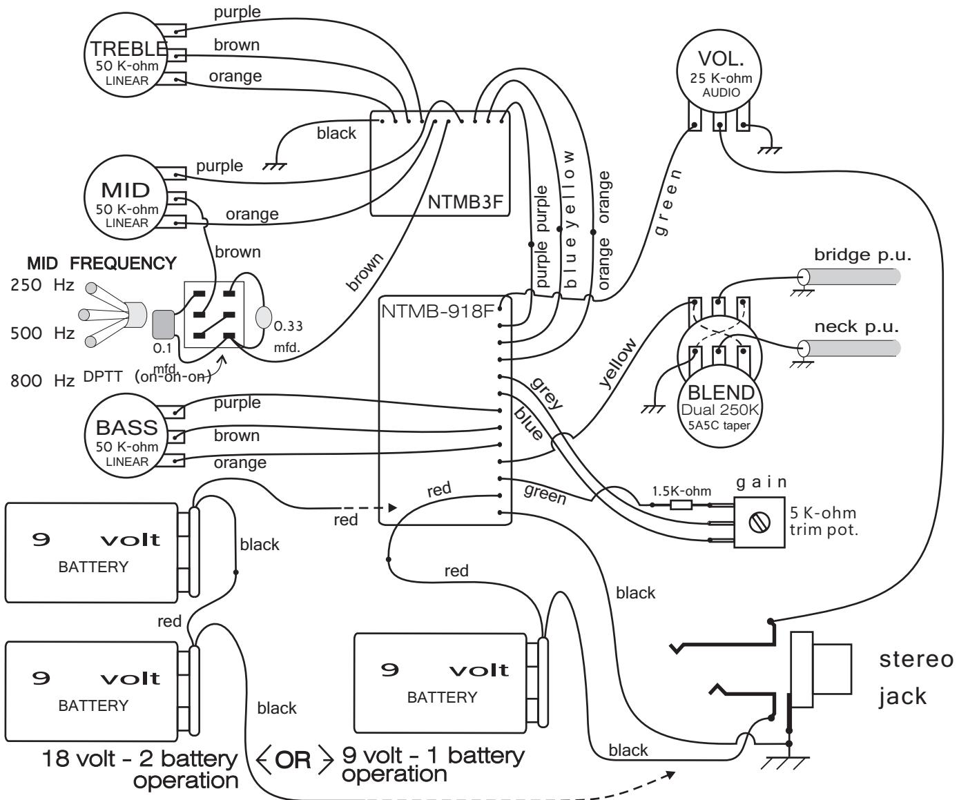
The NTMB is a tone control preamp with fully independent Bass, Mid and Treble controls with very low noise and wide boost/cut range. It consists of 2 prewired modules for ease of installation.
