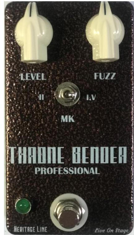
The Throne Bender Germanium Fuzz features two control knobs and a toggle switch:
